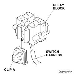
49. Install the relay to the switch harness relay block.
