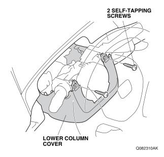
12. Remove the lower column cover (one self-tapping screw).
