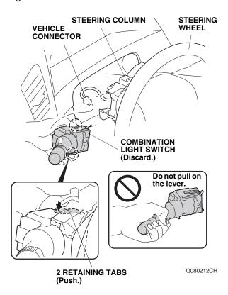
57. While pushing the two retaining tabs, slide the combination light switch out and remove it from the steering column.
