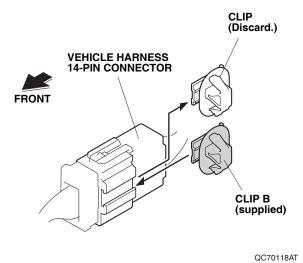
43. Unplug the vehicle harness 14-pin connector.
