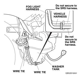
29. Under the washer tank, secure the fog light harness to the vehicle harness with one wire tie as shown. Do not secure the fog light harness to the SRS harness.
