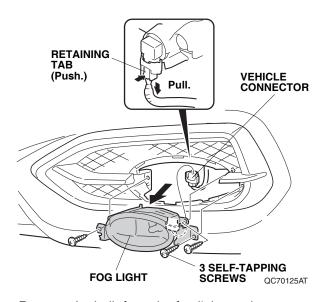
3. Remove the bulb from the fog light as shown.
