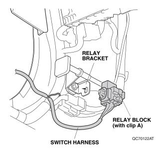
51. Plug the switch harness 4-pin connector and 6-pin connector into the fuse box. Go to step 54.
