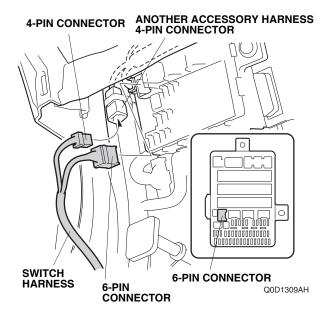
54. Secure the switch harness to the vehicle harness with two wire ties.
