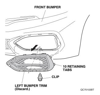
17. Install the new left fog light trim to the front bumper with 10 retaining tabs and 1 clip.
