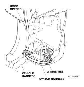
55. Secure the switch harness to the vehicle harness with two wire ties.
