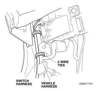
56. Unplug the vehicle connector from the combination light switch.
