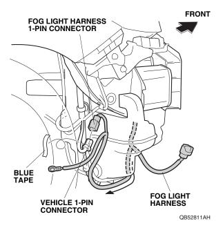
23. Plug the fog light harness 1-pin connector into the vehicle 1-pin connector as shown.
