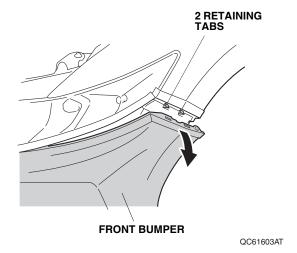
On each side, release four retaining tabs.
