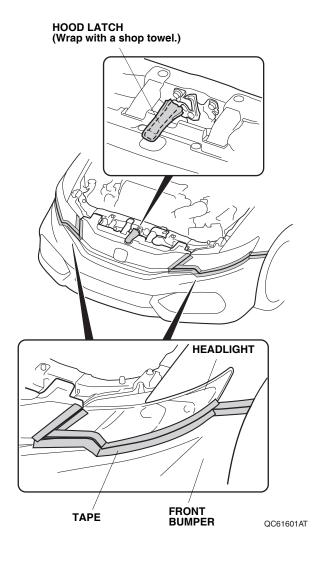
• Remove the 4 self-tapping screws, 10 clips, and 2 bolts.
