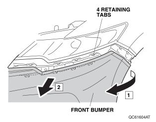
With the help of an assistant, remove the front bumper (four clips). Place the front bumper on a blanket to prevent damage.
