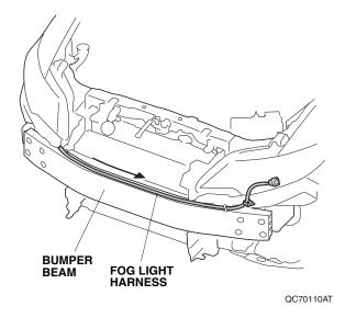
34. Secure the fog light harness clip to the hole in the extension as shown.
