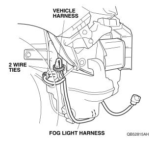
28. Secure the fog light harness to the vehicle harness with two wire ties as shown. Do not secure the fog light harness to the SRS harness.
