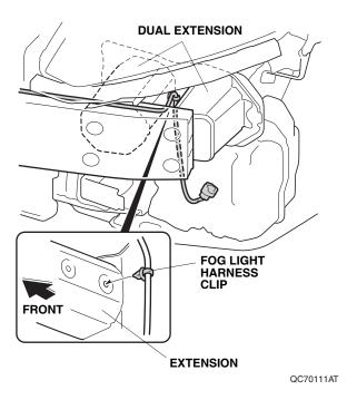
35. Using isopropyl alcohol on a shop towel, clean the bumper beam where the aluminum tapes will attach.
